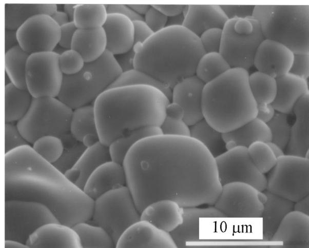
Figure 4 SEM micrograph of a stoichiometric composition of perovskite  $\text{Pb}(\text{Mg}_{1/3}\text{Nb}_{2/3})\text{O}_3$  heat treated at  $900^\circ\text{C}$  for 3 h showing a near single-phase microstructure.
