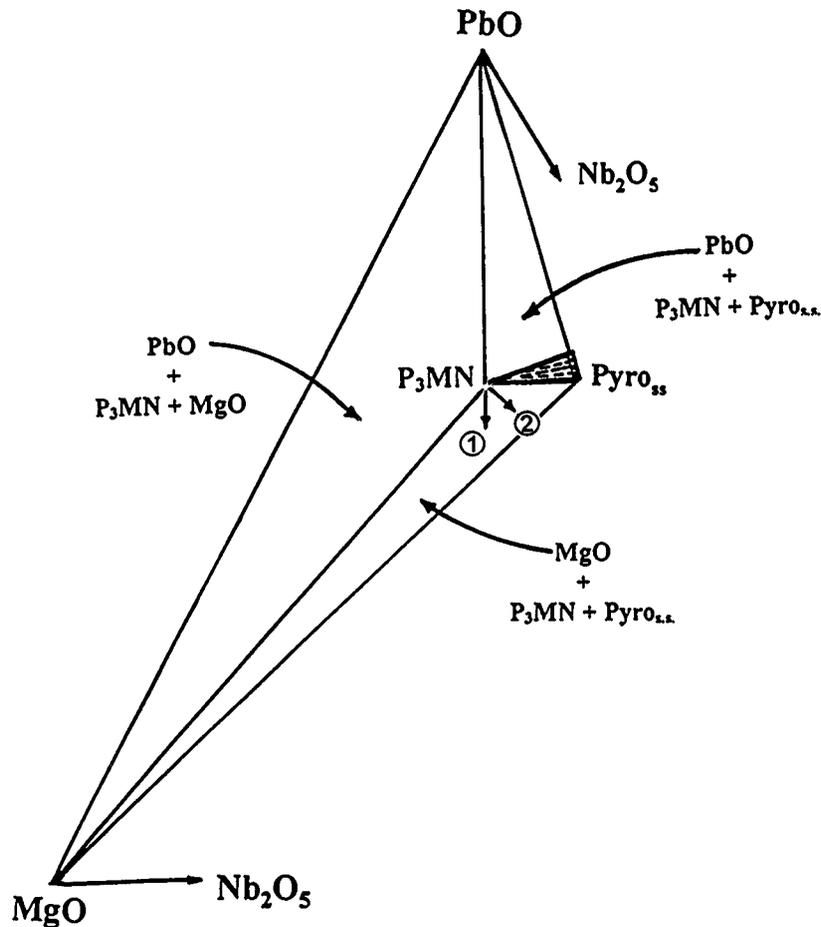
Figure 8 Partial phase diagram of the ternary system PbO-MgO-Nb<sub>2</sub>O<sub>5</sub> showing the subsolidus compatibility relations between the various phases at 800 °C (P<sub>3</sub>MN = perovskite Pb(Mg<sub>1/3</sub>Nb<sub>2/3</sub>)O<sub>3</sub> and Pyro<sub>s.s.</sub> = Pyrochlore solid solutions).
