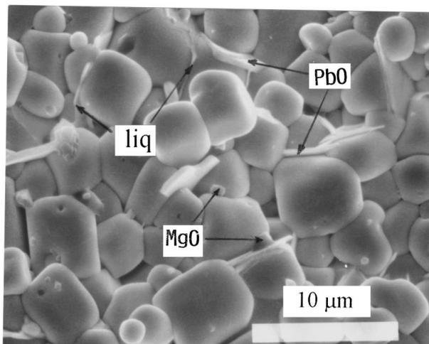
Figure 3 SEM micrograph of a stoichiometric composition of perovskite  $\text{Pb}(\text{Mg}_{1/3}\text{Nb}_{2/3})\text{O}_3$  heat treated at  $850^\circ\text{C}$  for 3 h showing melt formation and crystallization of PbO in the grain boundaries.
