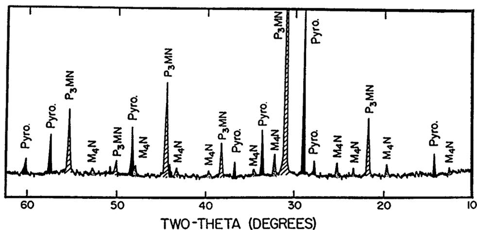
Figure 5 X-ray powder diffraction pattern of a diphasic mixture containing perovskite  $\text{Pb}(\text{Mg}_{1/3}\text{Nb}_{2/3})\text{O}_3$  and the pyrochlore phase which was partially melted at  $1250 \text{ }^\circ\text{C}$  showing the formation of  $\text{Mg}_4\text{Nb}_2\text{O}_9$  ( $\text{P}_3\text{MN}$  = Perovskite  $\text{Pb}(\text{Mg}_{1/3}\text{Nb}_{2/3})\text{O}_3$ , Pyro = Pyrochlore phase, and  $\text{M}_4\text{N}$  =  $\text{Mg}_4\text{Nb}_2\text{O}_9$ ).
