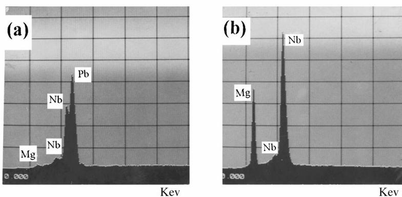
Figure 7 EDX patterns of different grains of the ternary pyrochlore composition (a) sintered grain of phase-pure pyrochlore phase, (b) solid grain that formed after partial melting at  $1250^\circ\text{C}$ .
