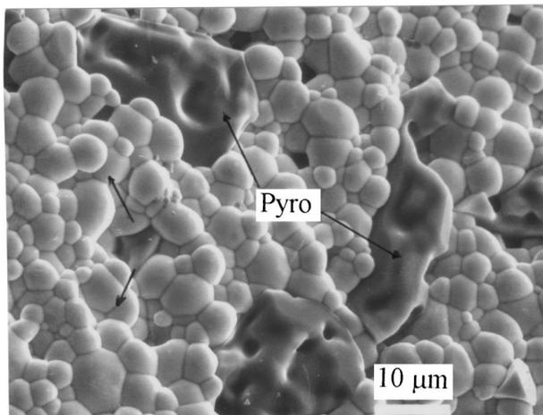
Figure 6 SEM micrograph of a diphasic mixture containing perovskite  $\text{Pb}(\text{Mg}_{1/3}\text{Nb}_{2/3})\text{O}_3$  and the ternary pyrochlore phase showing the onset of melting of the pyrochlore phase at  $1250^\circ\text{C}$ .
