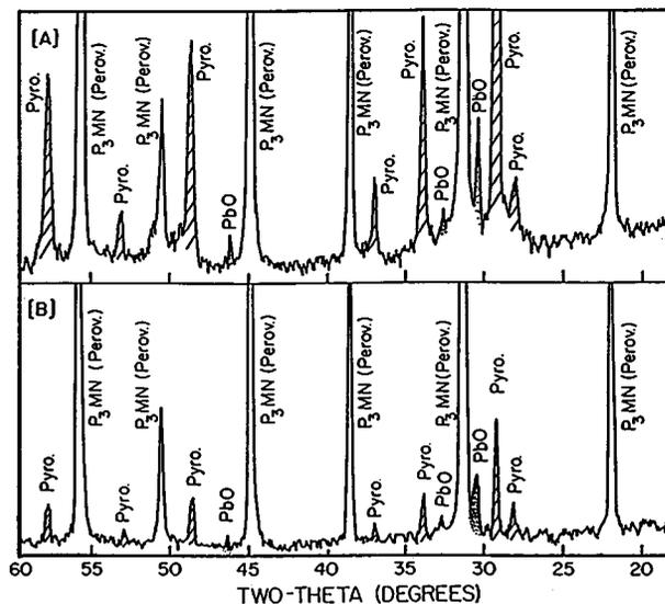
Figure 1 X-ray powder diffraction patterns of a stoichiometric composition of perovskite  $\text{Pb}(\text{Mg}_{1/3}\text{Nb}_{2/3})\text{O}_3$  heat treated for 3 h at (A) 750 °C and (B) 800 °C.
