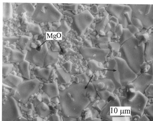
Figure 2 SEM micrograph of a stoichiometric composition of perovskite  $\text{Pb}(\text{Mg}_{1/3}\text{Nb}_{2/3})\text{O}_3$  heat treated at 750 °C for 3 h showing the distribution of various reaction products.
